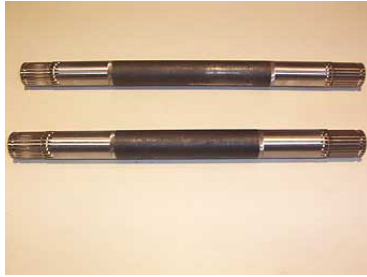
Better design: unspliced axle shafts.
