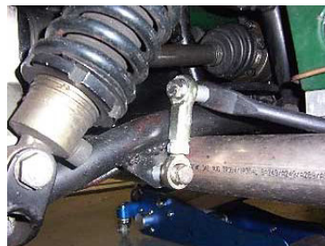
The Heim joints facilitate side-to-side adjustment. There is actually more clearance here than it appears!
