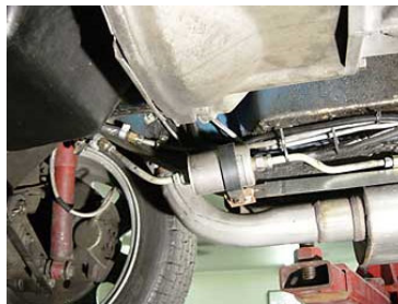
Driver-side of fuel tank, and fuel pump mounting Fuel filter & EFI line connections to engine & return line to old MGB line
