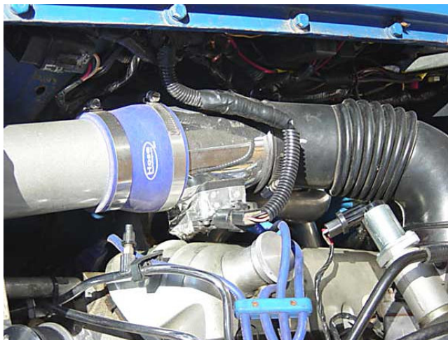
MAF sensor (PMAS brand) and cold air intake tube.
