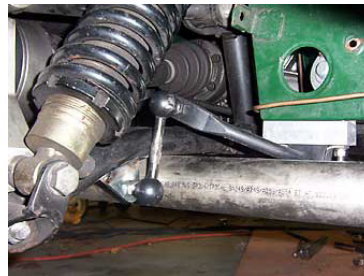
They worked... but I decided to replace them with adjustable links. Advantage: increased stiffness from eliminating the rubber ends.
