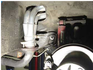
Passenger-side header & oxygen sensor
