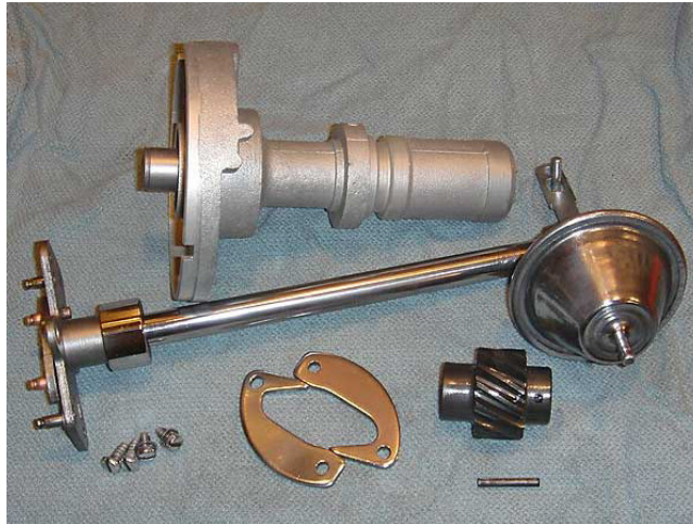
Photo 1: Buick 215 Distributor, Cleaned Up and Torn Down
