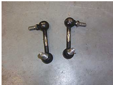
MG Midget attachment links were cut and re-welded. The welding must be done carefully (quickly) to avoid melting the rubber!
