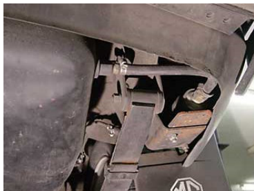
Driver-side of fuel tank, and fuel pump mounting Fuel filter & EFI line connections to engine & return line to old MGB line
