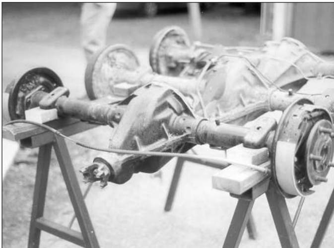
Jeep Dispatcher Dana 44 rear ends (two in front) and MGB (rear) Simple spring mounts on Dana are easily replaced with salvaged or new MGB mounts.
