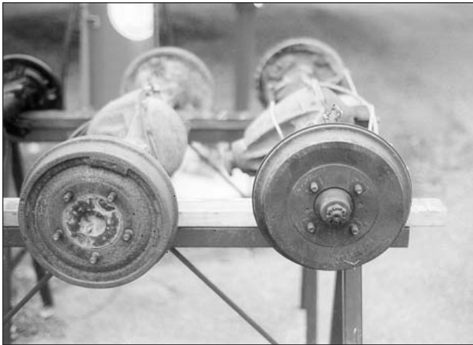
Dana (L) and stock MGB (R). Note that the Dana axle end is flat between the lug nuts. The undesirable AMC version of the Jeep rear end has a protruding nut at the axle end, just like an MGB, making identification easy.
