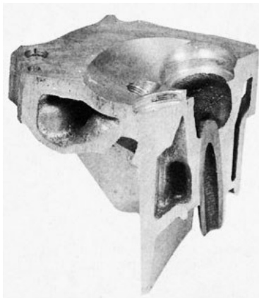
Spark plug boss is water-cooled as are valve guides. Special press fit holds guides in place. Removal of manifold reveals embossed sheet metal valve cover doubling as manifold gasket. Pad at top of cover prevents drumming, aids silencing.
