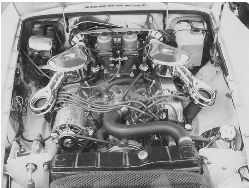
The Rover 3.5-litre V8, surely the most versatile engine that has yet been built.
